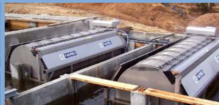
View on 2 filters 32-160 with frame in sturgeon farm
