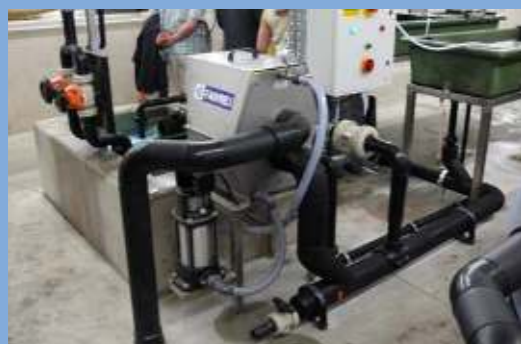
Model 2-40 with 36µ mesh on recirculation system.
