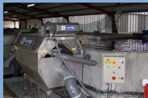
Model 4-80 with 36µ mesh on recirculation system.
