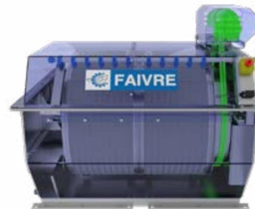
Rotoclean 80 drum filters benefit from the BDS system (Belt Drive & Support system). The motor, ideally placed on top of the drum filter, drives and supports the drum with one or more belts.
