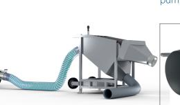
Hopper with water separator for loading tanks Ref.: **TD0801**
