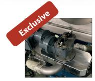
Electrically operated 4 - way valve allowing precise control of the closing speed of the valve. Your fish are safely transported.
